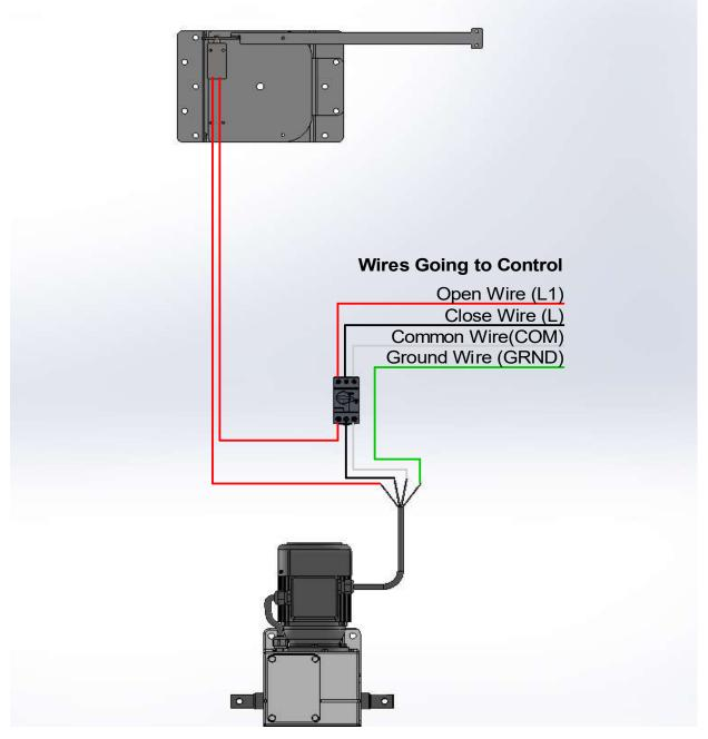
240v power needed. Refer to control wiring diagram for instructions to connect into the control. Make sure you take open wire through the pulley as it will cause damage if not wired as per instructions.
